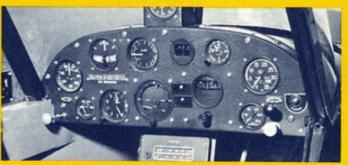
ADAPTABLE PANEL. The standard instrument group in the Super Cub includes altimeter, airspeed, compass, oil pressure and temperature gauge and tachometer. There is ample room in the full-size panel for complete instrumentation and radios. Dual flight and engine controls are standard, as are dual brakes.
