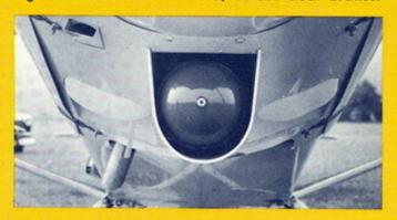
CARBURETOR HEAT AND FILTER. Carburetor heater and filter are standard Super Cub equipment. The air filter is of the new, improved paper type—99.5% effective, and easy and inexpensive to replace. This feature is of particular importance in the many Super Cubs operated under extremely dusty conditions.
