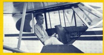
CONVENIENT CABIN. The Super Cub's front seat is adjustable fore and aft. To enlarge the space available for cargo, the rear seat can be quickly and easily removed. For photography, hunting of predatory game, and other special purposes, the hinged right door and window can be opened in flight. An abundant supply of warm air is regulated by means of a cabin heat control and left hand windows have panels to admit cool fresh air.
